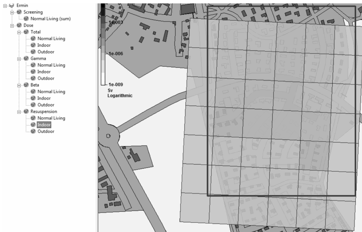
Figure 2. A screen shot from the ARGOS Emergency DSS, showing the visualisation of ERMIN results against background map of an urban area.
